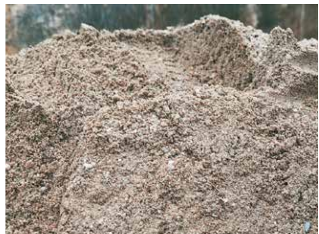
Washed grit removed at a wastewater treatment plant.
