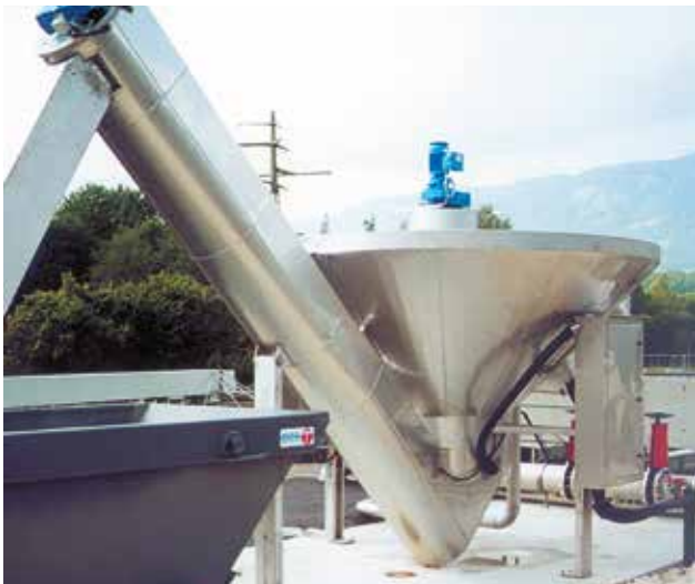
Innovative technology: HUBER Coanda Grit Washer RoSF4 size III with frost protection for outdoor installation.
