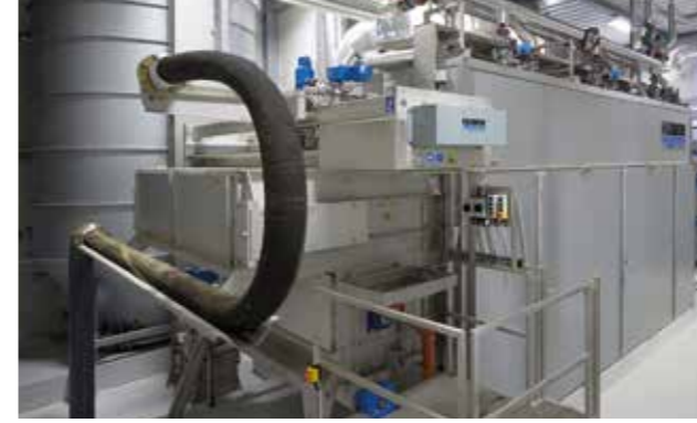
Sludge feeding with HUBER extruder unit (pelletizer).
