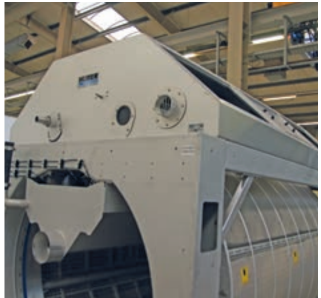
Polyurethane sealing in the inlet of the HUBER Drum Screen LIQUID.
